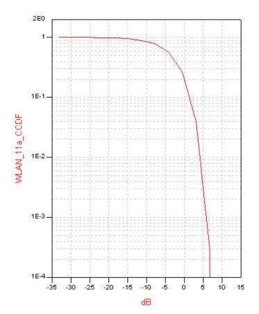
In <u>CCDF Curve for WLAN 802.11a 54 Mbps Signal</u>, you can see that the instantaneous signal power exceeds the average signal power (0 dB) for 20% of the time. You can also see that the instantaneous signal power exceeds the average signal power by 5 dB for only 0.3% of the time.
