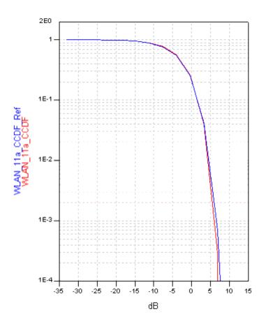
CCDF Curve for WLAN 802.11a Signal with Reference Curve
